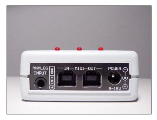
In the left side of the panel where is written "Analog Input", usually you can connect some kind of analogue source. For example: a breath controller, foot pedal, potentiometer and etc. Polarity of connecting of the input connector is showed in the picture.
